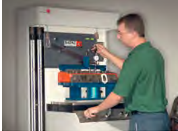
High Performance Racing Technology instructor Steve Davenport, uses the flow meter to evaluate the components that flow air into and out of the engine in an effort to increase the efficiency of the engine.
